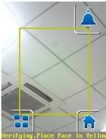
Note: the recognition interface has three buttons: clicking the button in the top right corner can output the doorbell; clicking the key in left bottom can enter into the System Management menu; clicking the key in right bottom can return to the main interface.
