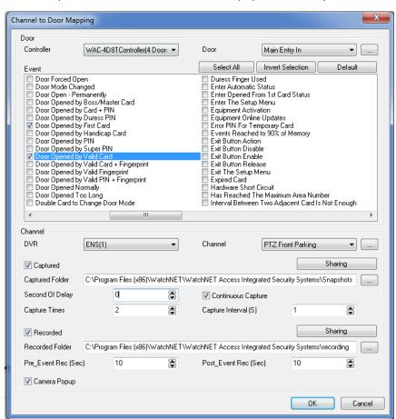
Note: in order for the Recorded to work the DVR has to be setup for 24 hour recording.
